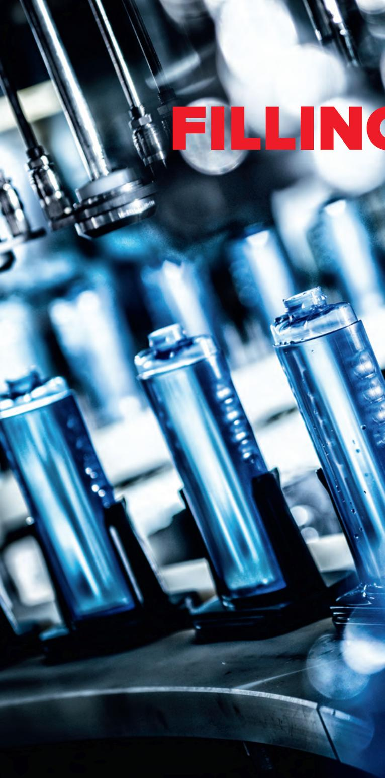
Always at the same level. Our Tölke experts have developed the Voluminizer. When filling a bottle, the Voluminizer ensures that nothing foams or overflows. No matter how high the filling level is, the Voluminizer always fills with the same distance to the fill level. This saves you annoying cleaning of overflows. And speaking of saving: Our filling machine can be changed over quickly and easily.
